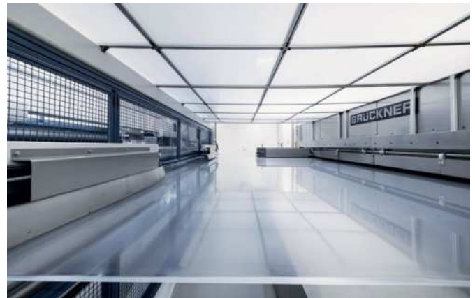
Battery separator film production line_Brückner Maschinenbau
